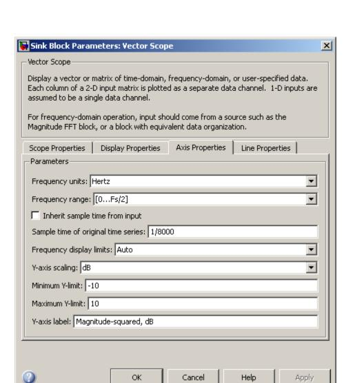
Because you are buffering the input with a nonzero overlap, you have altered the sample time of the signal. As a result, you need to specify the sample time of the original time series. Otherwise, the overlapping buffer samples lead the block to believe that the sample time is shorter than it actually is.
