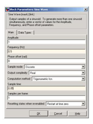
**Note** On Signal Processing Blockset blocks, the **Sample time** parameter represents the sample period of the signal. The sample period is the amount of time between each sample of the signal.
