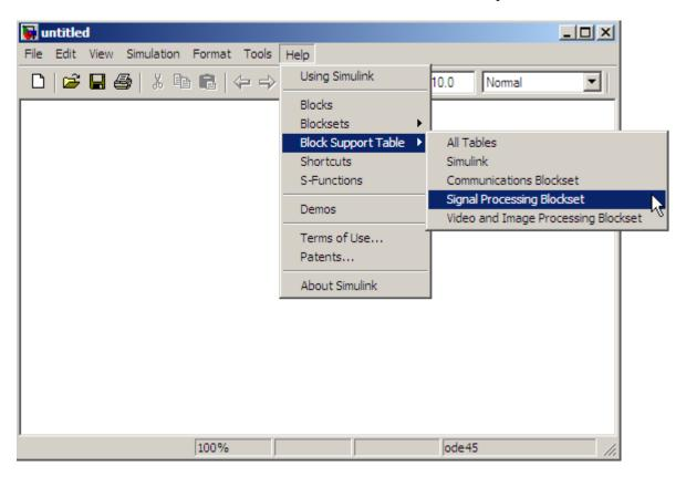
You can also access the Signal Processing Blockset Data Type Support Table by typing showsignalblockdatatypetable at the MATLAB command line.
