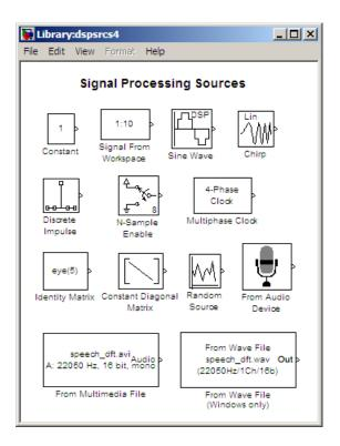
4 Click-and-drag a Sine Wave block into your new model. The Sine Wave block generates a sinusoidal signal.
