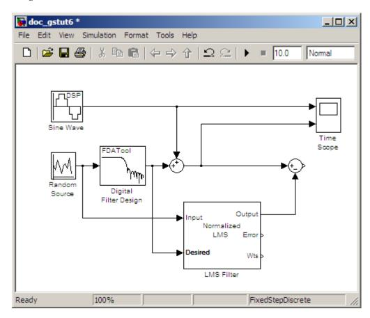
The positive input to the second Sum block is the sum of the input signal and the low frequency noise, s(n) + y. The negative input to the second Sum block is the LMS Filter block's best estimation of the low frequency noise, y'. When you subtract the two signals, you are left with an approximation of the input signal.
