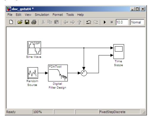
**3** Run your model and view the results in the Time Scope window. This window shows the original input signal and the signal with low frequency noise added to it.
