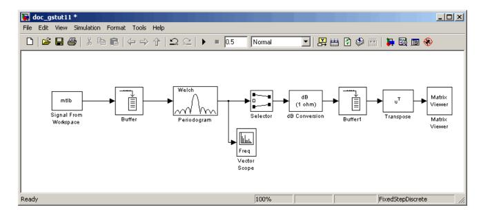
Once you have assembled the blocks needed to view the spectrogram of your speech signal, you can set the block parameters.
