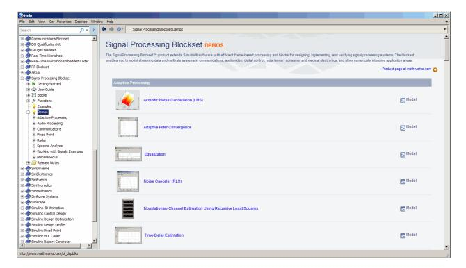
**3** To view the description of the Equalization demo, which demonstrates adaptive channel equalization, expand **Adaptive Processing** then click **Equalization**.
