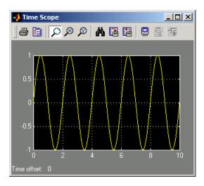
**5** Experiment with your model. Change the **Frequency (Hz)** and **Sample time** parameters of the Sine Wave block. Then, run your model to see the effect. Now you are ready to add noise to your sinusoidal signal and view its effect.
