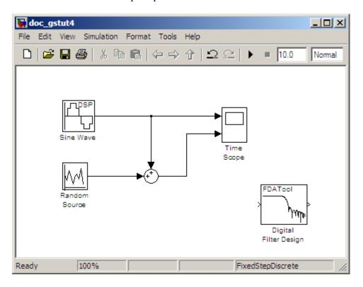
**2** Incorporate the Digital Filter Design block into your block diagram by placing it between the Random Source block and the Sum block.
