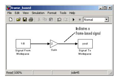
To have the Signal From Workspace block output a frame-based signal, set the **Samples per frame** parameter to 2 and run the model. The lines that connect the blocks become double lines, indicating a frame-based signal; in this example, there are two signals per frame.
