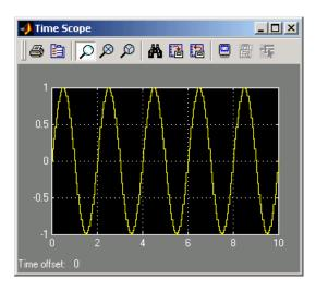
You can achieve a more finely sampled output by decreasing the **Sample time** parameter. For example, change the **Sample time** parameter in the Sine Wave block to 0.005, run the model, and autoscale the output. The Time Scope window should now look similar to the following figure.
