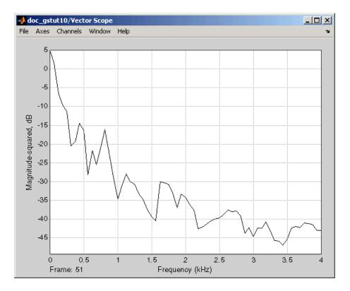
During the simulation, the Vector Scope window displays a series of frames output from the Periodogram block. Each of these frames corresponds to a window of the original speech signal. The data in each frame represents the power spectrum, or contribution of every frequency to the power of the original speech signal, for a given window.
