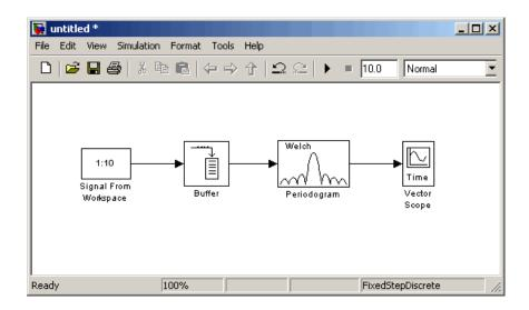
Once you have assembled the blocks needed to calculate the power spectrum of your speech signal, you can set the block parameters.
