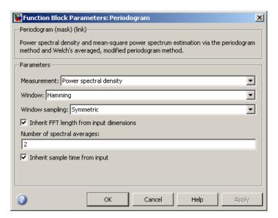
Based on these parameters, the block applies a Hamming window periodically to the input speech signal and averages two spectra at one time. The length of the FFT is assumed to be 128, which is the number of samples per frame being output from the Buffer block.
