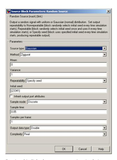
Opening this dialog box causes a running simulation to pause. See "Changing Source Block Parameters During Simulation" in the online Simulink documentation for details.
