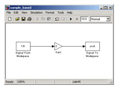
The Signal From Workspace block outputs a sample-based signal. The Gain block multiplies all the samples of the signal by two. Then, the Signal To Workspace block outputs the signal to the MATLAB workspace in a variable
