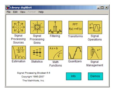
**2** Open a new model by selecting **File > New > Model** in the Signal Processing Blockset library window.
