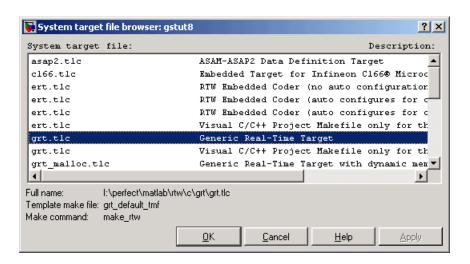
The **Real-Time Workshop** pane now displays the correct system target file (grt.tlc), make command (make\_rtw). and template makefile (grt default tmf).
